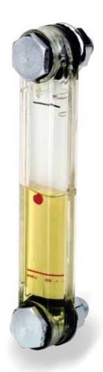
Thermoplastic level gauges made from transparent polyamide which provides good mechanical resistance and is impervious to mineral oil, gasoline, lubricants, petroleum, solvents and most chemical agents (please refer to technnical table N.1 page 58); avoid contact with alcohol based solutions and antifreeze liquids at high temperatures and hot water over 80°C
