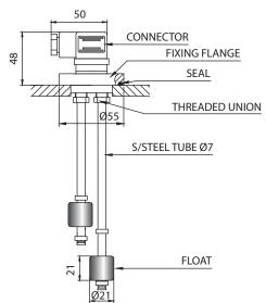
Insert the wires and tube in the threaded union located under the flange, then suitable tighten for perfect assembly. Connect the connector to the flange and the respective wires to the base, and the level indicator is ready to use.
