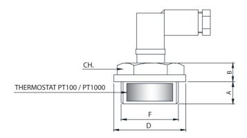
The temperature probe occupies the space provided for every common drain plug for tanks, control units, oil sumps, etc.
