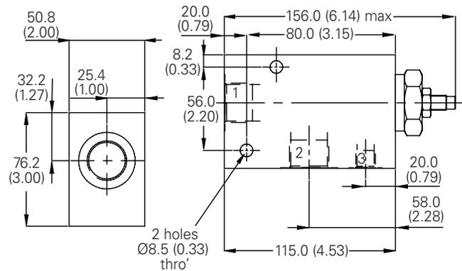
Note. Tightening torque of "F" adjuster locknut - 20 to 25 Nm
